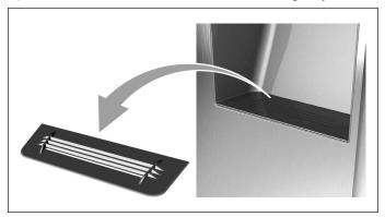
■ To clean the water collecting tray and the strainer, the strainer can be taken out.
