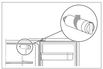
Screw in the water filter in clockwise direction and make sure it is firmly fitted to the water filter base.
