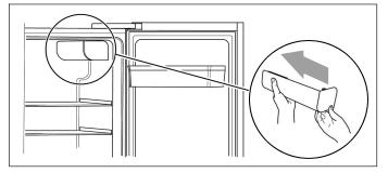
5. Reattach the filter cover by gently sliding it on.
