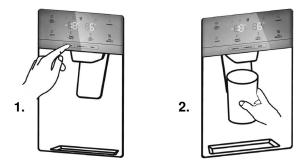
1. Press button "cubed ice" or "crushed ice" to activate dispenser mode "cubed ice" or "crushed ice".
