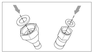
2. Install the two pads to the hose nuts.
