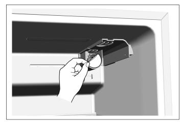
3. Remove the protector of the water filter base.
