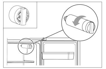
2. Screw out the old water filter in anticlockwise direction (see sign on the filter) and remove it.
