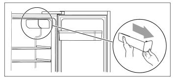
1. Open the refrigerator door to its maximum angle and remove the water filter cap by pulling it out slowly.
