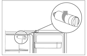
**4.** Screw in the water filter in clockwise direction and make sure it is firmly fitted to the water filter base.
