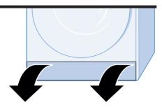
Release the lever in the heat exchanger cover and pull it out by the handle.
