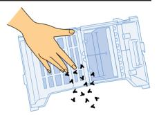
Rinse the empty fluff collector under running water and dry it.
