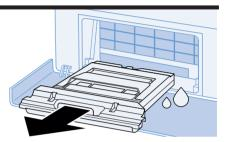
Open the fluff collector and remove any fluff.
