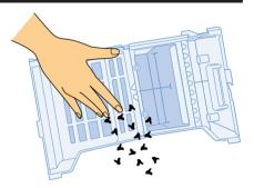
Rinse the empty fluff collector under running water and dry it.
