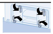
Remove all fluff from the cover thoroughly and remove the fluff filter.
