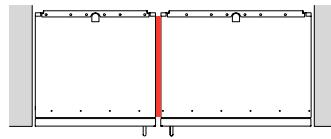
EN: When the appliances are installed less than  $6\frac{1}{4}$ " (160 mm) apart from one another, but not connected side-by-side, purchase the heater kit **HEATRKIT20** (Freedom Heater Kit). This kit is also recommended for use with any installation in areas that are subject to extreme humidity.
