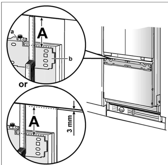
2. Desapertar as 2 porcas (a) e retirar a barra de ajuste (b).
