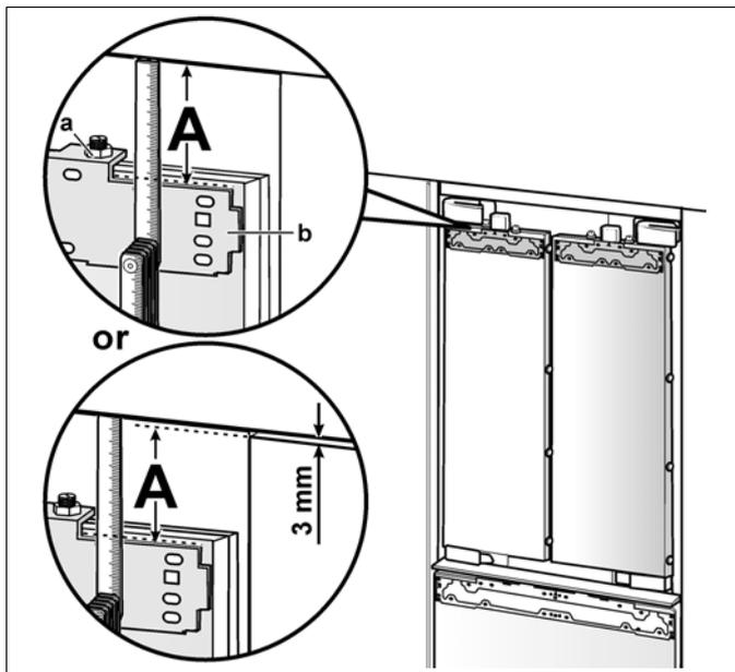
2. Desapertar as 2 porcas (a) e retirar a barra de ajuste (b).
