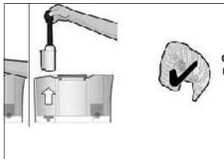
**i** Rinsing the filter simultaneously activates the setting for displaying the message "Please change water filter". When this message appears, or at the latest after two months, the filter will no longer be effective. It needs to be replaced for reasons of hygiene and to prevent a build-up of limescale (which could damage the appliance).
