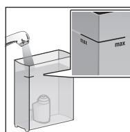
Now remove the water tank and fill it with cold water up to the "max" mark.
