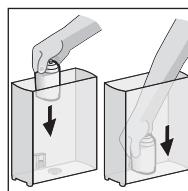
Then place the filter cartridge firmly in the water tank by hand (or using the measuring spoon if you have it nearby).
