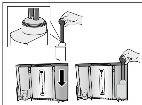
4. Fill the water tank with water up to the "max" marking.
