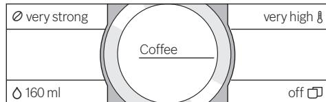
**i** There are different setting options depending on the type of drink. For coffee drinks, for example, the strength, temperature and quantity can be set, for milk only the volume.
