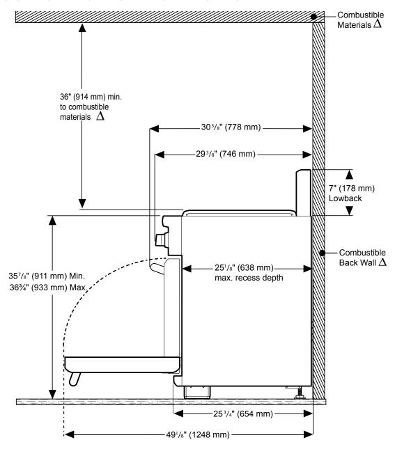
$\Delta$  As defined in the "National Fuel Gas Code" (ANSI Z223.1, Current Edition). Clearances from non-combustible materials are not part of the ANSI Z21.1 scope and are not certified by CSA. Clearances of less than 6" (152 mm) must be approved by the local codes and/or by the local authority having jurisdiction.
