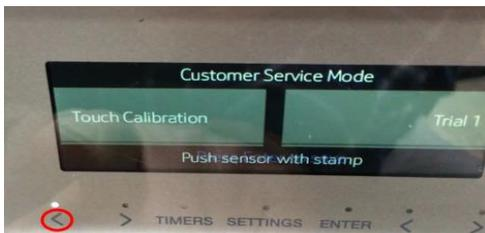
3. Release pressure from finger when display shows Release Sensor. Then move to the next button as display prompts.
