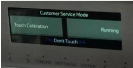
2. Start calibrating once display reads as below Touch Calibration ~Trial 1 mode and Push Sensor with finger or stamp and Release Sensor with stamp. *Pressing too hard may affect the Button Test to time out.* Touch and hold once first < button on left illuminates. Remove your finger when the a beep is heard and light goes out. (See following next step)
