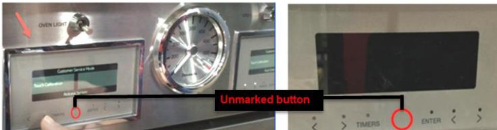
In Pro ranges with two User Interfaces, the right User Interface is used for activating Customer Service Mode. The aux steam oven display calibrates the same as the main display except on that display it has Drawer on the Display Setting.
