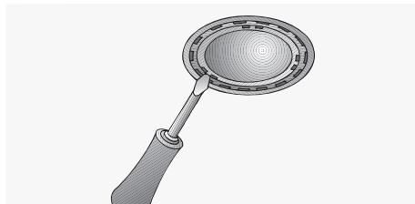
3. Replace the halogen light bulb (conventional halogen bulb, 12 Volt, max. 20 Watt, G4 cap).
