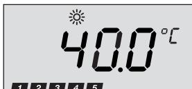
The continuous-flow heater can be operated with pre-warmed water (for example from a solar energy unit). The "Symbol Sun" will appear in the display if the feed water temperature is above 30 °C.
