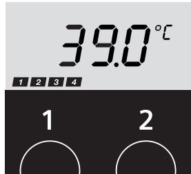
Both programs will repeat until either the **button 1** or **2** is pressed (depending on the program selected) or the water faucet is shut off for more than 2 minutes or the temperature setting is changed. The temperature which was set before the program was started will be re-activated.
