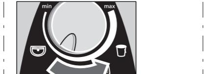
If a higher temperature for a completely opened warm water tap is not achieved, more water flows than the flow-through heater can warm as a result its performance capabilities. In this case, the warm water tap must be closed somewhat.
