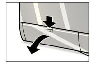
☐ Take the drainage hose out of the holder and pull out of the housing.
