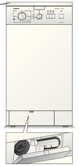
Drain washing solution if necessary
