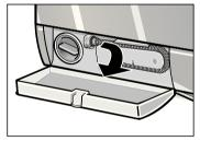
☐ Remove the sealing cap and drain the water into a receptacle.
