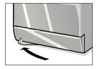
Swivel the lever under the front of the appliance from right to left. The appliance is now standing on its rollers.
