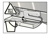
Press on the sealing cap and insert the drainage hose into the holder.
