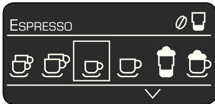
The status line **5a** in the display shows the name of the type of drink, along with the strength setting, e.g. **00** and per-cup quantity, e.g. **□**. The selection line **5b** shows symbols for the drink selection. The arrows in the navigation line **5c** indicate the direction in which more menu levels can be found.
