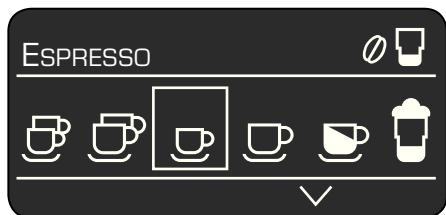
The status line **5a** in the display shows the name of the type of drink, along with the strength setting, e.g.  $\emptyset\emptyset$  and per-cup quantity, e.g.  $\square$ . The selection line **5b** shows symbols for drink selection. The arrows in the navigation line **5c** indicate the direction in which more menu levels can be found.
