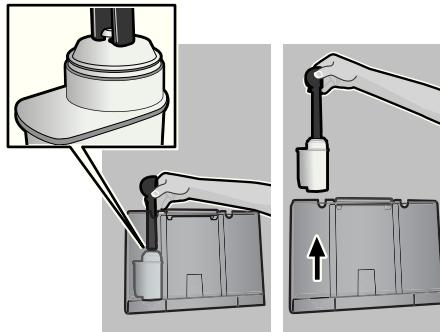
**Note:** Rinsing the filter **34** simultaneously activates the setting for the "change filter" display.
