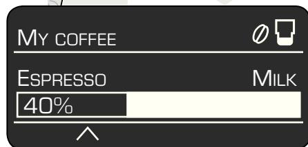
In addition to selecting the coffee strength and per-cup quantity you can choose the exact mix of espresso and milk for your own coffee setting MY COFFEE <sup>1</sup>. The setting can be defined in 20% steps by turning the rotary knob **6**.
