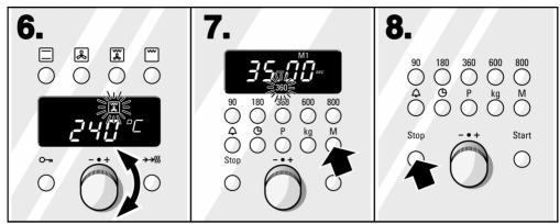
**6.** Set the temperature to 240 °C using the temperature selector.
