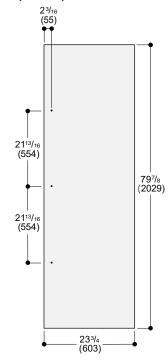
The door panel thickness is  $^3$ / $_4$ " (19 mm) The maximum door panel dimensions are based on a clearance of  $^1$ / $_8$ " (3 mm), based on a single niche
