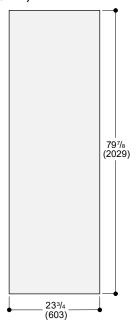
The door panel thickness is  $^3/^4$ " (19 mm) The maximum door panel dimensions are based on a clearance of  $^1/_8$ " (3 mm), based on a single niche
