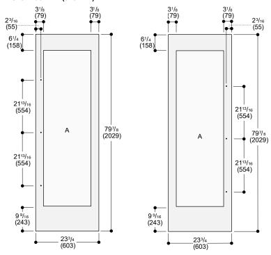
The door panel thickness is 3/4" (19 mm)
