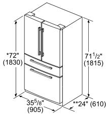
\*Add  $^{5}$ /8" (17) with front leveling feet fully extended
