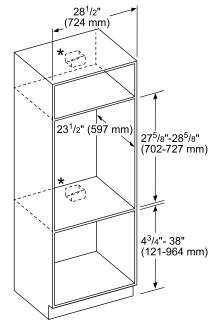
\* For single ovens installed into a wall cabinet, the junction box may be located above, beneath, left or right of the unit within reach of the power cord.
