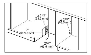
NOTE: Plumbing installations will vary—refer to local codes. The maximum length of the drain hose, including hose leading to air gap (if any) is 150" (380 cm). Ensure a portion of the drain hose is raised at least 33" (84 cm) above the floor to ensure proper draining
