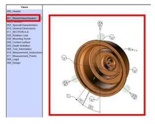
If extension lines of PMIs are hidden by geometry, switching the model render mode to "Transparent" could be helpful
