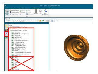
By selecting a specific model view, users can now access the prepared dynamic PMI model views. The interaction is facilitated through standard mouse functions.
