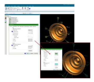
By Change of the "Foreground" color of both the "Text" and the "Geometry" the PMI coloring will be changed.
