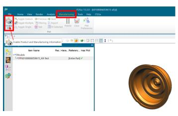
There are multiple ways available to display the PMIs, which are organized in specific model views. The suggested approach for single part involves right-clicking on the geometry to access the desired information.
