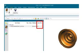
Furthermore, please ensure that the application PMI is enabled in the ribbon "Manufacturing". Fortunately, this is a necessary one-time action.
