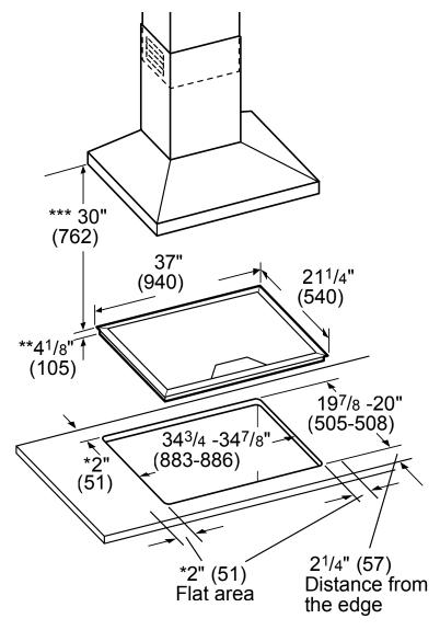
**NOTE:** The work surface should be horizontal and level. The stability of the countertop should be confirmed even after making the cutout.
