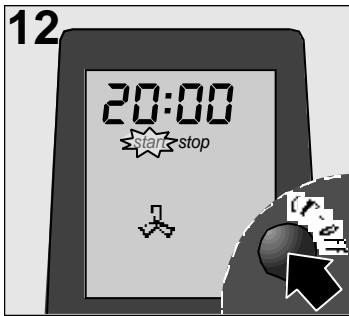
□ Press the < or > button in order to alter the timer setting. The timer is set in blocks of 15 minutes.
