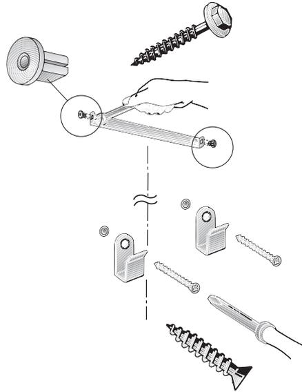
7. Attach the extractor hood. Adjust the height and align horizontally with the adjusting screws.
