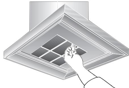
3. Insert the metal grease filters.
