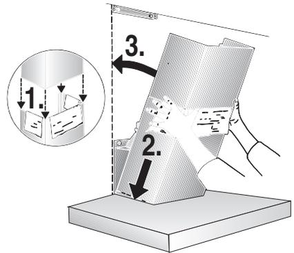
13. Slide out the upper section and attach it to the mounting brackets at the sides with two screws.
