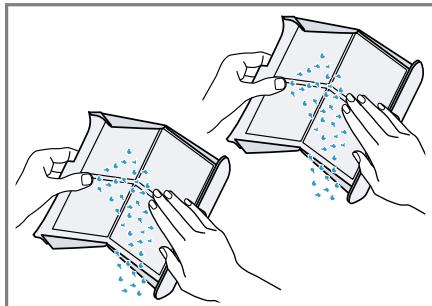
**8. Sita za vlakna očistite temeljno mlažom tople vode i osušite ih.**
