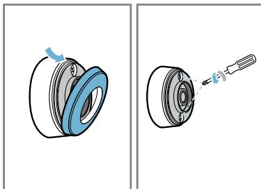
2. Open the cooking sensor cap and remove the battery from the base.
