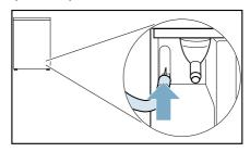
Take the drain hose from the accessories and attach it to the free socket, pushing it up to the stop.
