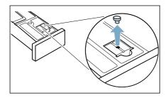
3. Turn the condensation container 180° onto its underside and insert the stopper.
