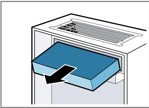
**2.** Insert the new odour filter into the circulating-air module.
