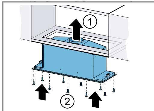
2. Tighten the fastening screws.
