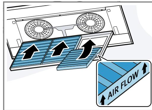
Insert the odour filter in the correct direction.
