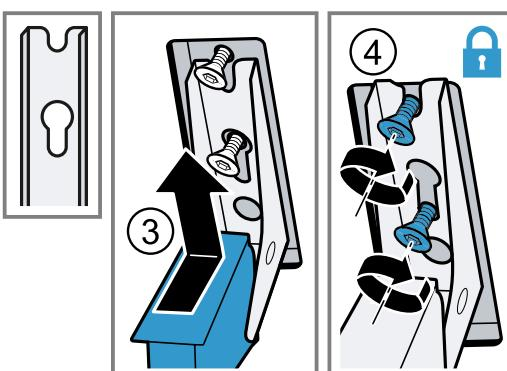
**3. Tighten the fastening screws on the hinges.**
