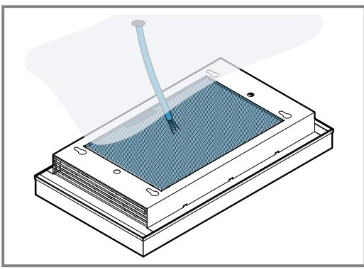
3. Guide the cable that is provided on-site through the opening and hook the appliance into the fastening screws on the ceiling.
