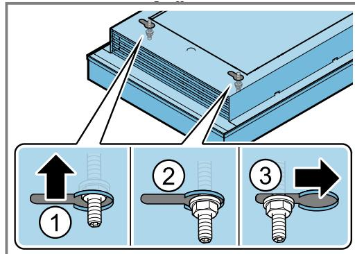
6. Carefully tighten the diagonally opposite collar nuts until the appliance is flush-mounted on the ceiling.
