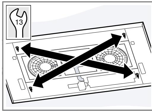
Tighten the collar nuts one at a time so that the appliance does not tilt when doing so.
