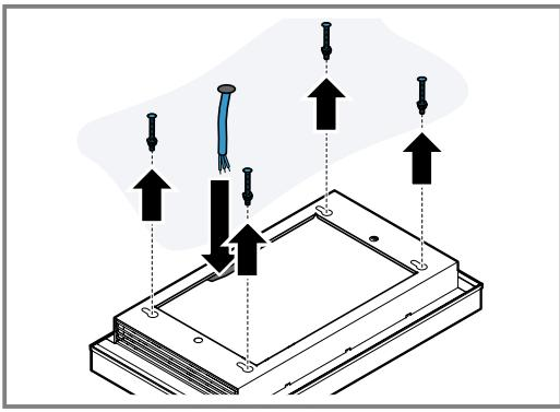
4. Push the appliance as far as it will go into the four key hole openings using the guide sleeves.
