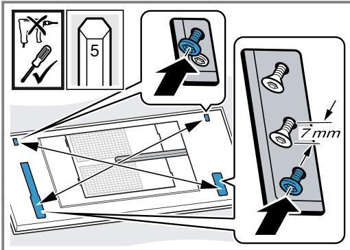
Tighten the screws one at a time so that the appliance is not wedged in the cut-out.
