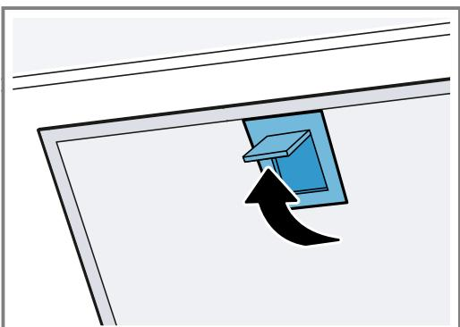
4. Remove the grease filters from the holders.
