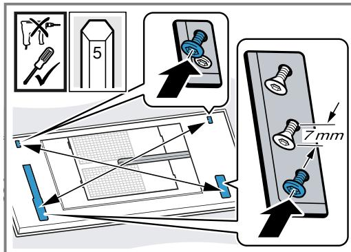
Retighten the screws if necessary.
