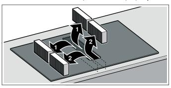
Insert two of the activated charcoal filters or acoustics filters into the left and right of the appliance and slide them forwards.
