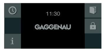
The child lock is activated. The standby screen appears. The  $\Box$  symbol is shown at the top of the display.
