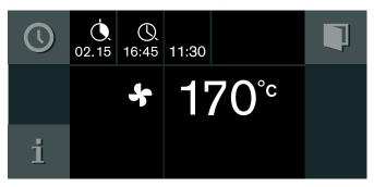
The appliance switches to standby. The heating mode, temperature, cooking time and cooking time end appear in the display. The appliance starts at the calculated time and switches off automatically when the cooking time has elapsed.
