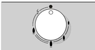
For dual double flame burners, the inner and outer flames can be controlled separately.
