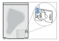
5. Take the drain hose from the accessories and secure it to the free connecting piece.
