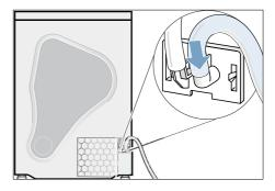
6. Fasten the other end of the drain hose with the remaining accessories, depending on the connection situation (A, B or C).
