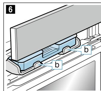
9. Slowly push the control panel downwards and then towards the rear until it is closed completely.
