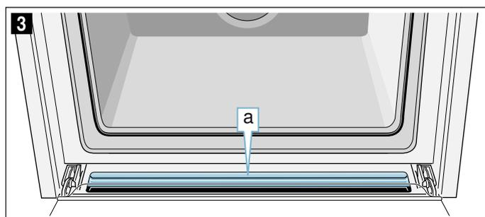
**Note:** If the seal has become detached, fit the seal back onto the drip trough. → "Appliance door" on page 31
