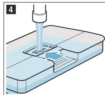
7. Reinsert the cover **a** into the opening in the water tank.
