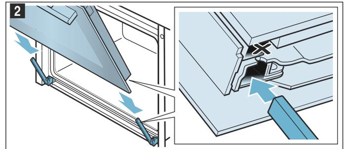
3. Open the appliance door fully. Close the two locking levers (figure 3).
