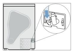
5. Take the drain hose from the accessories and secure it to the free connecting piece.
