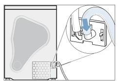
**6.** Fasten the other end of the drain hose with the remaining accessories, depending on the connection situation (A, B or C).
