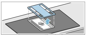
2. Take the metal grease filter and the container out.
