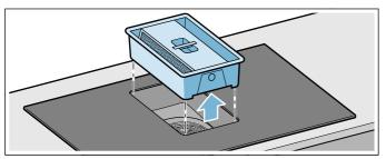
**Note:** Fat may accumulate in the bottom of the container. Hold the metal grease filter level to prevent grease from dripping out.
