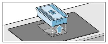
**3.** Press down on the catches on either side of the container to separate the metal grease filter from the container.
