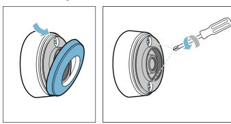
2. Open the closure of the temperature sensor. Remove the battery from the lower section of the housing and insert a new battery (pay attention to the correct orientation of the battery poles).
