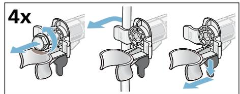
3. Insert the covers. Lock the covers firmly in place by applying pressure to the snap-in hooks.
