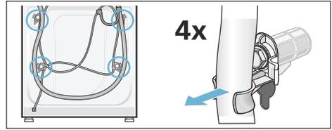
2. Unscrew and remove all four transportation securing bolts with a wrench (WAF 13). Remove the sleeves. Remove the mains cable from the holders.
