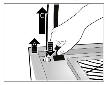
5. Once you have repositioned the appliance, use an open-ended spanner (WAF 7) to tighten the turnbuckles.
