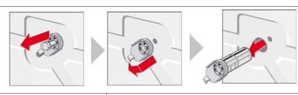
Unscrew all screws using the spanner supplied.
