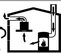
Room air-dependent heat-producing appliances (e.g. gas, oil, wood or coal-operated heaters, continuous flow heaters or water heaters) obtain combustion air from the room in which they are installed and discharge the exhaust gases into the open air through an exhaust gas system (e.g. a chimney).
