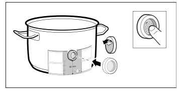
Press the silicone patch down, including its inside surface.
