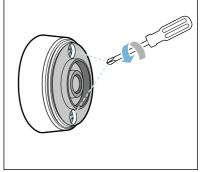
2. Remove the upper section of the casing. Take the old batteries out. Put the new batteries in. Make sure that the polarity is correct.
