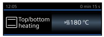
The » \$\mathbb{M}\$ symbol appears on the left next to the temperature. The temperature indicator starts to fill in.
