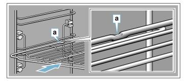
When inserting baking trays, ensure that the catch tappet  ${\bf a}$  is at the rear and is facing downwards. The sloping edge of the accessory  ${\bf b}$  must be facing forwards towards the appliance door.
