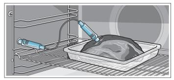
**Poultry:** Insert the meat probe as far as it will go into the thickest point in the breast. Insert the meat probe into the poultry crossways or lengthways depending on its structure. Then turn the poultry and place it on the wire rack breast-side down.
