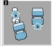
3. Use the hook to attach the rear holder into the upper hole **a** and push it into the lower hole **b** (fig. **3**).
