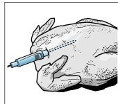
**Turning the food:** If you wish to turn the food, do not remove the meat probe. Once you have turned the food, check that the meat probe is correctly positioned in the food.
