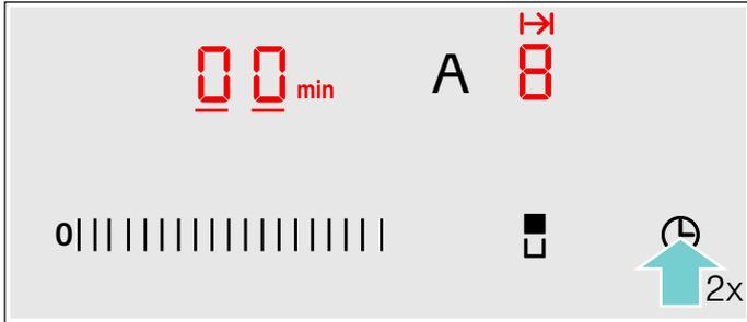
3. Touch the desired presetting in the settings range. The possible presetting from left to right is 1, 2, 3, etc., to 10 minutes. Within 10 seconds, slide your finger along the settings range repeatedly until the desired cooking time is reached.
